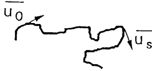
FIGURE 2 Worm like trajectory for the photons in a scattering medium.
